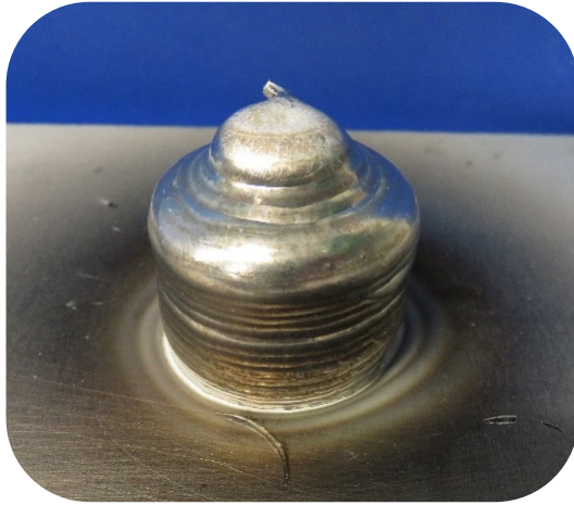
EBAM material deposited on the build plate
