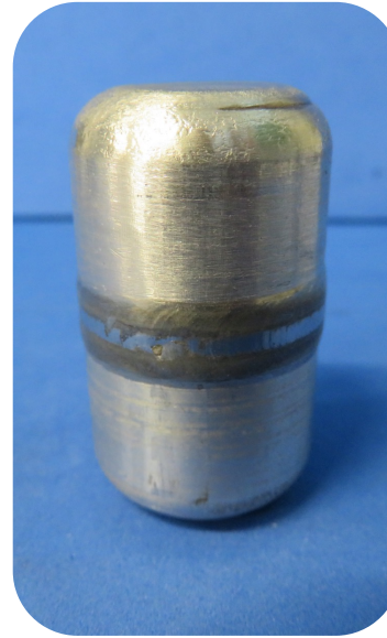
Finished demonstrator fabricated by EB welding
