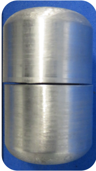
Pre-weld assembly of two EBAM parts
