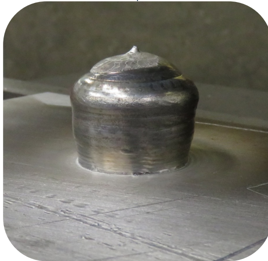
Material sinking at the center
